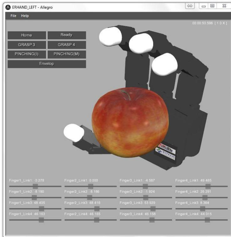
AHAS is provided along with the Allegro Hand for two main purposes. AHAS allows for ease of testing CAN communication between your PC and the Allegro Hand hardware. Secondly, AHAS provides several robust grasping algorithms for use with the Allegro Hand. The algorithms provided with AHAS can grasp a variety of object geometries for demonstration or for use at the end of a manipulator.
