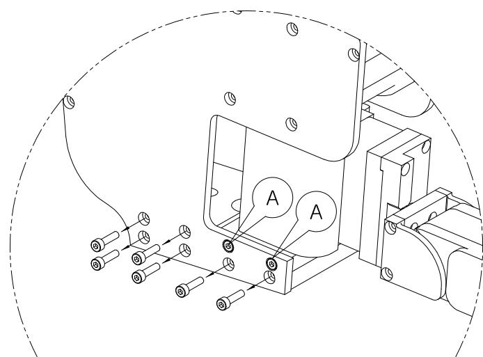
Once the twelve (12) screws have been removed, the mounting block can be removed from the bottom of the hand.
